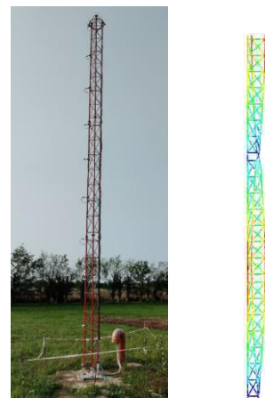
Left: Test structure in Ruthe; Right: Loaded FEM-Model
